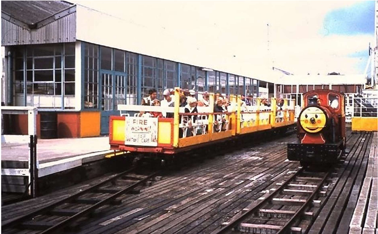
The locomotive is seen here running round a reasonably well-loaded three coach train at the shore end station. Note the track with the sleepers laid directly on to the Pier decking. ( L. Hodgkinson Collection. 1970s )
